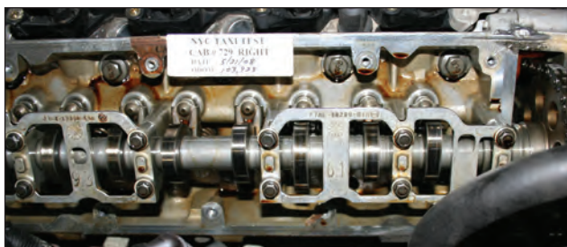
Poor quality motor oil, improper use of motor oil or neglected maintenance can all be to blame for the dirty valve deck above. Notice the difference with a clean valve deck if the proper oil is used and regular maintenance is followed.
